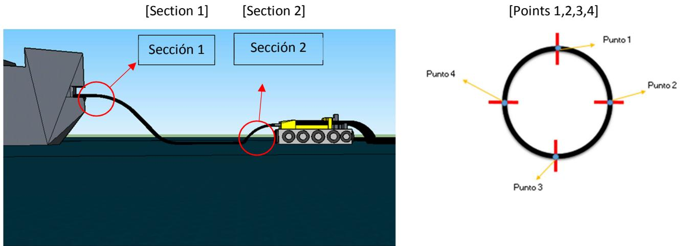
Figure No. 2.14: Measuring points for piping (ultrasound)
